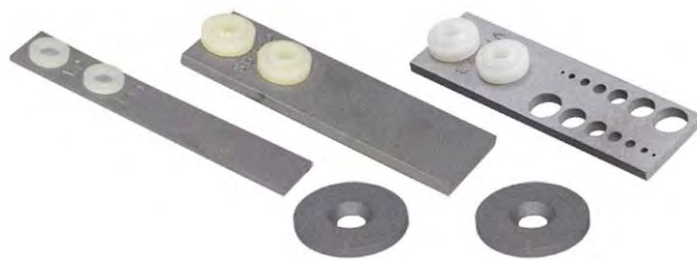
Figure 3-3. Example of corrosion coupons (image of Rohrback Cosasco System coupons, reprinted with permission).
