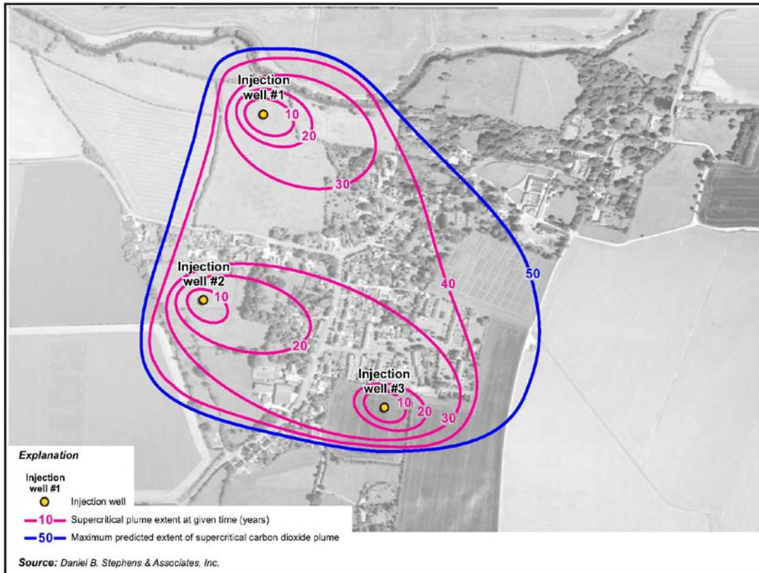
Figure 3-4: Hypothetical Geologic Sequestration Site: Model Predicted Extent of Supercritical Carbon Dioxide Plume Over Time
