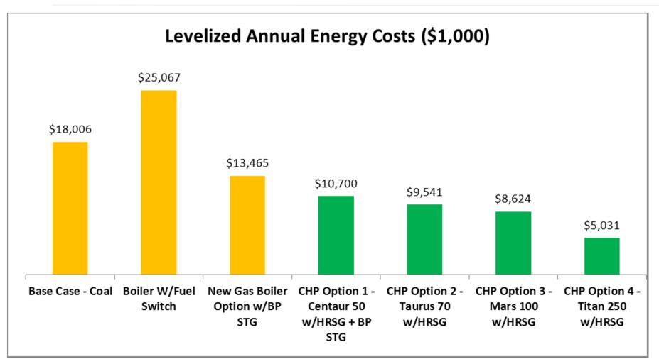
**Annual Energy Cost:** CHP Option 4 has the lowest annual energy cost compared to the other options. Energy Cost is offset by sale of excess or production of electricity for the larger CHP Option.
