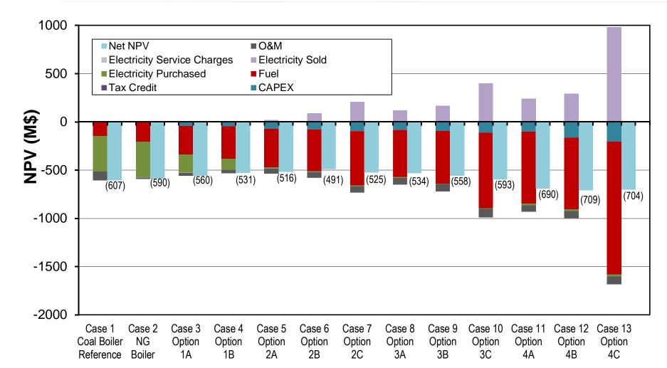
**NPV:** The Net NPV is lowest for LM6000 w/ back pressure steam turbine (Option 2B) Options 1B, 2A, 2C and 3A also had low NPVs. Therefore, these five CHP options are suggested for detailed analysis in a next step. **Eco**Nomics
