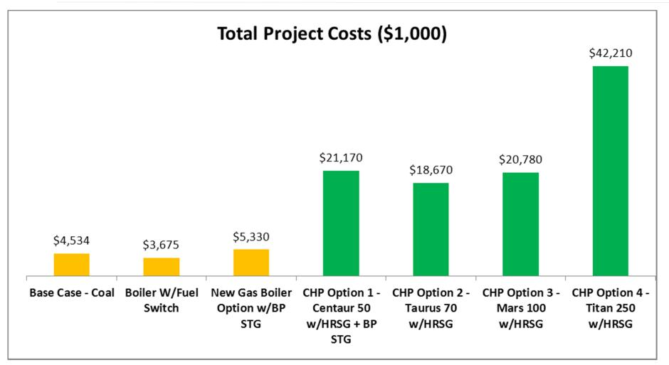
**Capex:** However, nothing comes free. The Gas Turbine CHP will cost between \$14 – \$38 million dollars more than the non GT CHP configurations. The higher delta for the GT based CHP also provides lowest energy cost. The GT CHP Capex includes 100% capacity back up NG Aux Boiler
