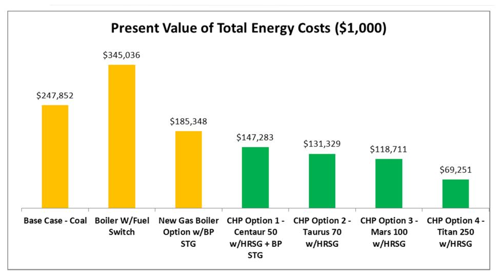
**NPV of Energy Cost:** The larger CHP option has lowest NPV of energy cost compared to the other options. Energy Cost is offset by sale of excess or production of electricity for the larger CHP Option.
