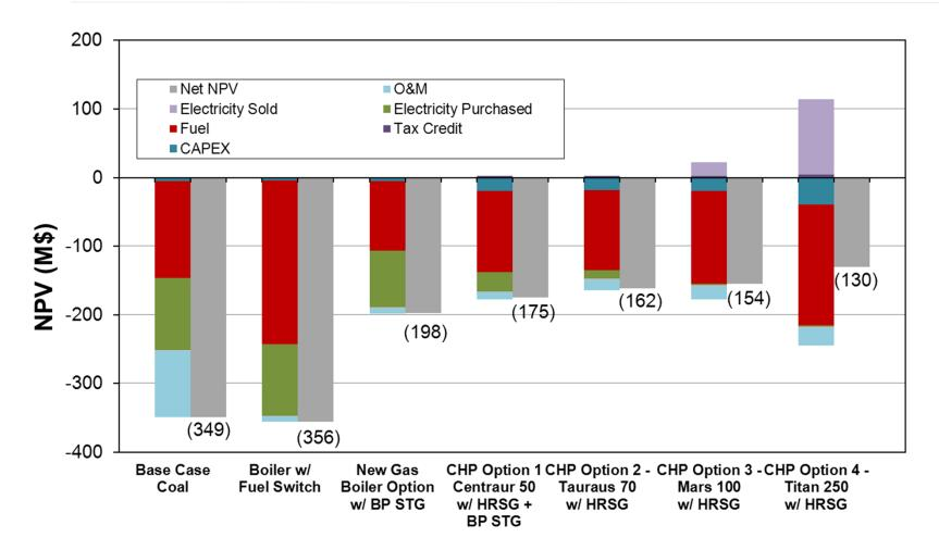
**NPV:** The Net NPV most positive for Option 4 with the larger CHP due to excess electricity sales. Base case and boiler fuel switch impacted by purchase electricity.
