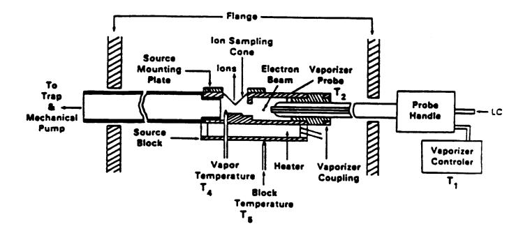
FIGURE 2 THERMOSPRAY SOURCE WITH WIRE-REPELLER (High sensitivity configuration)
