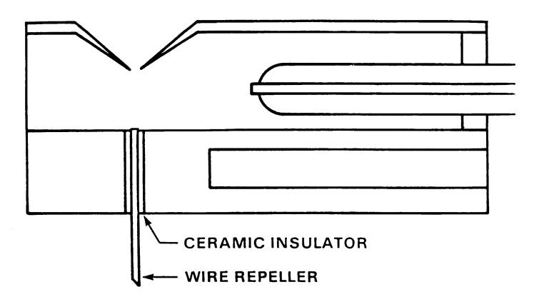
FIGURE 3 THERMOSPRAY SOURCE WITH WIRE-REPELLER (CAD configuration)
