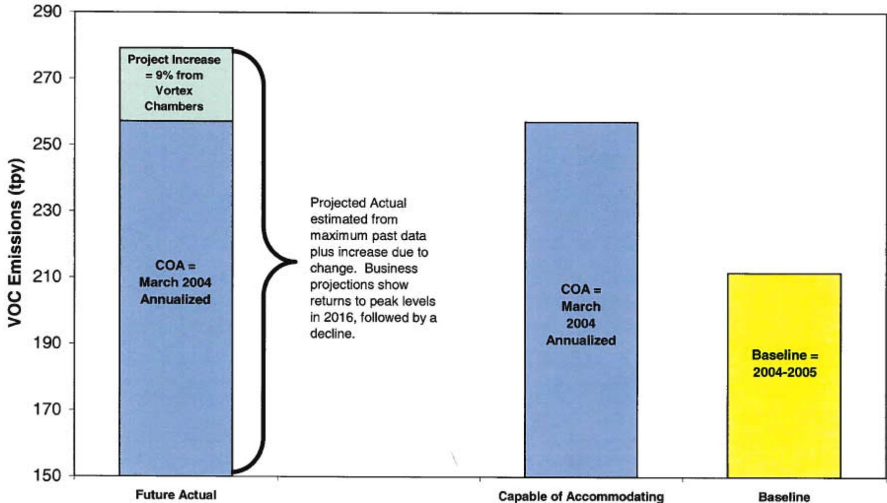
\*9% increase based on Kiln 3 modification (March 2009) which showed a potential for kiln batch times to decrease from 19 to 17.5 hours
