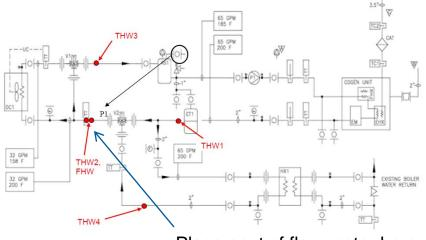
Placement of flow meter here would not capture UWHR
