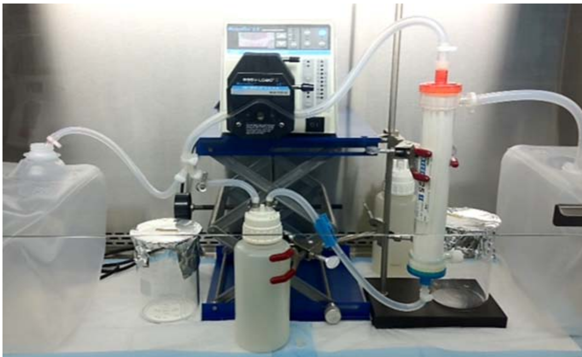
Figure 7b. Photograph of the ultrafiltration system set up inside a BSC.
