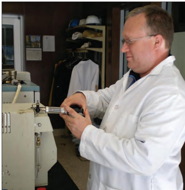
Figure 4-4. Lab Personnel Using Syringe to Inject GC.
