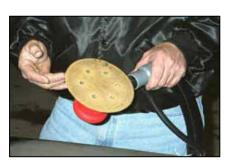
system. Use of a High Velocity Low Volume (HVLV) vacuum sanding system can protect workers and others nearby from harmful dust. When used and maintained properly, vacuum sanders can control 93-98% of the dust generated from the
