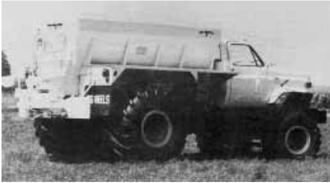
Figure 14-16. A 7.2-cubic-yard dewatered sludge spreader (courtesy of Big Wheels Inc.).
