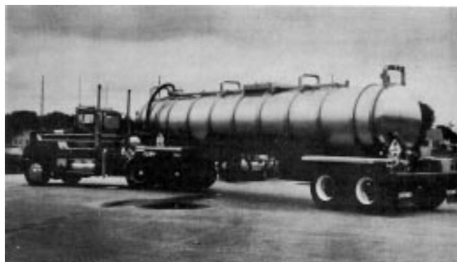
Figure 14-2a. A 6,500-gallon liquid sludge tank truck (courtesy of Brenner Tank Company).
