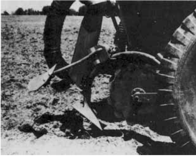
Figure 14-12a. Tank wagon with sweep shovel injectors (Cunningham and Northouse, 1981).
