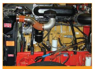
Membranes within the black housing mounted over the diesel engine pictured above generate NEA from cooled turbocharged air.
