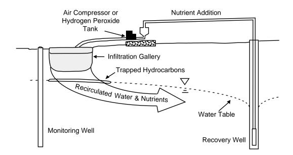
Figure 5. Use of infiltration gallery for recirculation of water and nutrients in in-situ bioremediation (Thomas and Ward, 1989).
