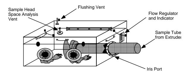
Figure 2. Field sampling glove box (Wilson, et al., 1989).
