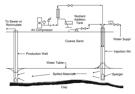
Figure 4. Typical schematic for aerobic subsurface bioremediation (Thomas and Ward, 1989).
