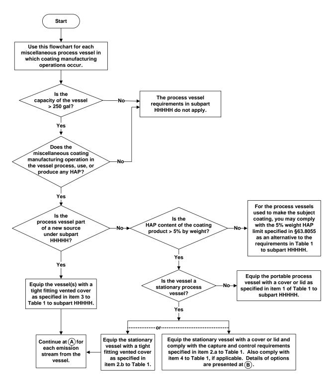
Figure 2. Flowchart of applicability and control requirements for process vessels.
