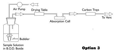
Figure 1. Apparatus for Flameless Mercury Determination
