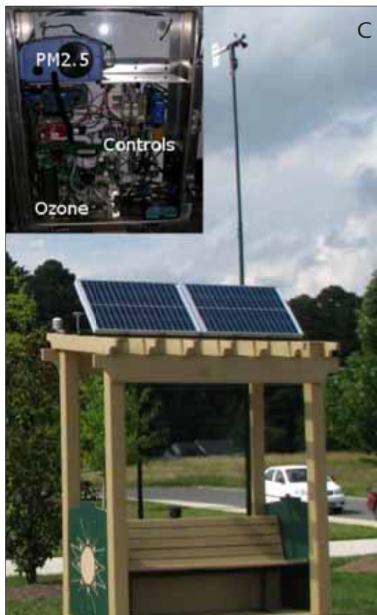
Figure 1. Example next-generation air monitoring systems. a) Portable M-Pod device that interfaces with a smartphone app (Photo credit: Ricardo Piedrahita); b) sensor network node during a forest fire emissions event (Johnson et al. 5 ); and c) Village Green Project—solar-powered and wirelessly transmitting community station, with inset image showing instrumentation enclosed in the bench structure.
