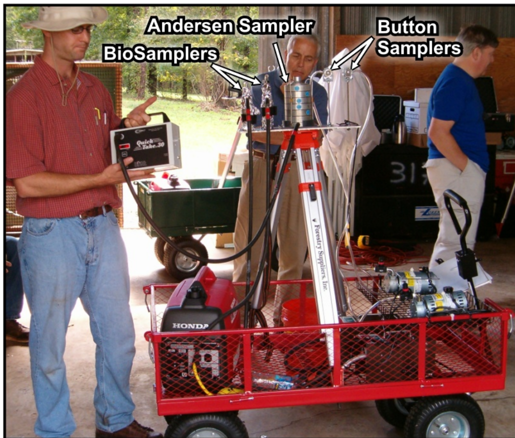
Figure 2-3. Cart-Mounted Transect Sampling Equipment
