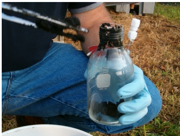
Figure 6-2. Glass Vessel Used for Biosolids Headspace Analysis
