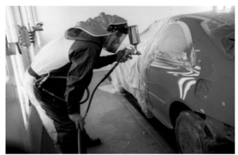
✤ By using a supplied-air, positive-pressure respirator, painters are much less likely to breathe harmful chemicals in paint spray. Most paint manufacturers say a supplied-air respirator is a Amust<sup>@</sup> when spraying highly toxic materials like isocyanates, the hardener in polyurethane clearcoats and in many primers. An air-purifying respirator will not provide adequate protection unless you develop and implement a proper filter change -out schedule, which can be a complex process.
