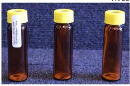
EPA Method 524.2 – Uses 40 ml clear vials (3 for samples, 2 for field blanks. Compounds: Volatile Organic Compounds (VOCs - Quantity: 89)
