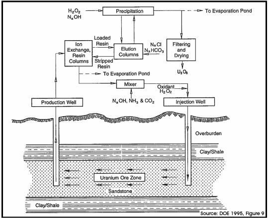
Figure 9: In-Situ Leach Uranium Recovery Flow Diagram
