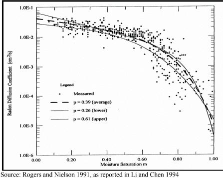
Figure 13: Diffusion Coefficient as a Function of Moisture Saturation
