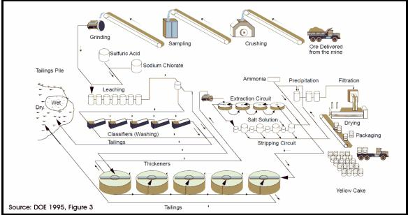
Figure 4: Typical Conventional Uranium Mill
