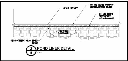
Source: Golder 2008, Drawing 8 Figure 24: Typical Double-Lined Impoundment with Leak Collection Layer
