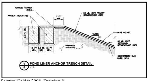
Source: Golder 2008, Drawing 8 Figure 25: Typical Double Liner Anchor System
