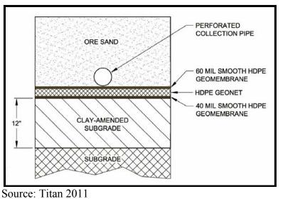
Figure 26: Typical Heap Pile Liner
