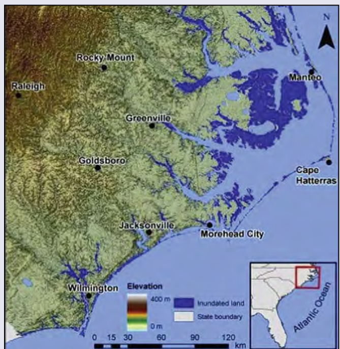
Figure 17. Dark blue shading represents land that is predicted to be under water with a 1-meter rise in sea level, expected in 65 to 200 years. Source: Poulter et al., 2009.
