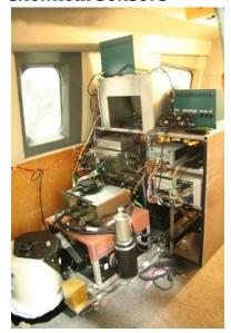
**Image 14:** View of chemical sensors: high speed infrared spectrometer, lower left corner; infrared line scanner is out of view behind the line scanner.
