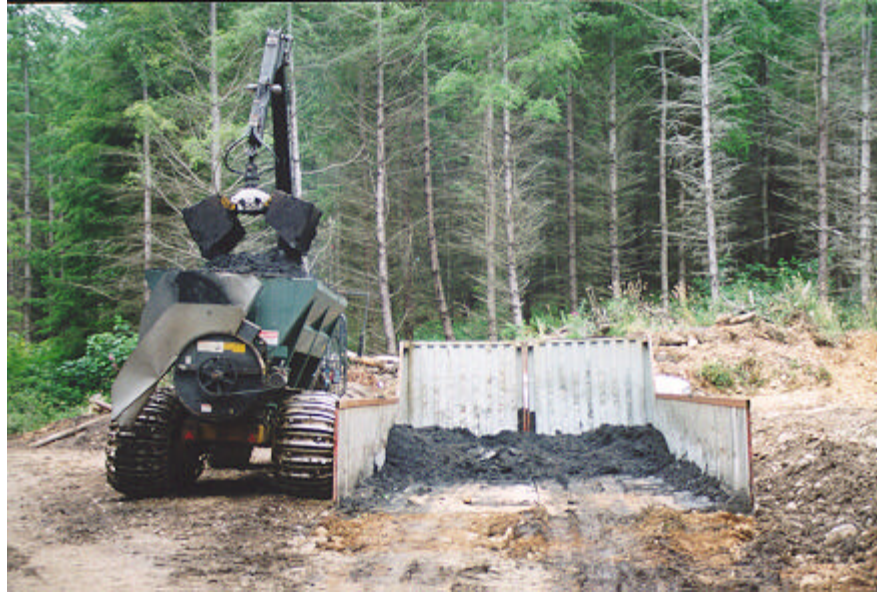
Figure 5-1. Daily biosolids deliveries are temporarily stored in a steel box fabricated from two intermodal freight containers (Snoqualmie Tree Farm, WA). The box breaks down and stacks together lengthwise for relatively easy relocation to the next unloading site. Biosolids are loaded from the containers into the Aero-Spread applicator by a clam bucket.
