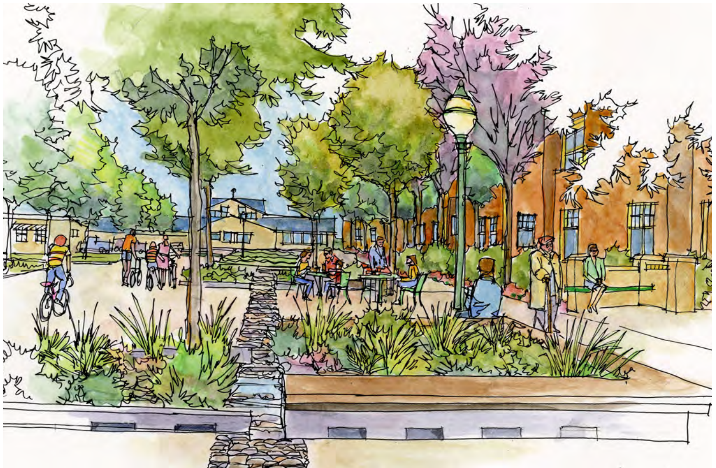
Figure 19: This design option depicts a shared street, providing flexible space where pedestrians, bicycles, and vehicles can use the same space. Landscaping and permeable paving help calm traffic, define where vehicles can be, and clean stormwater runoff.
