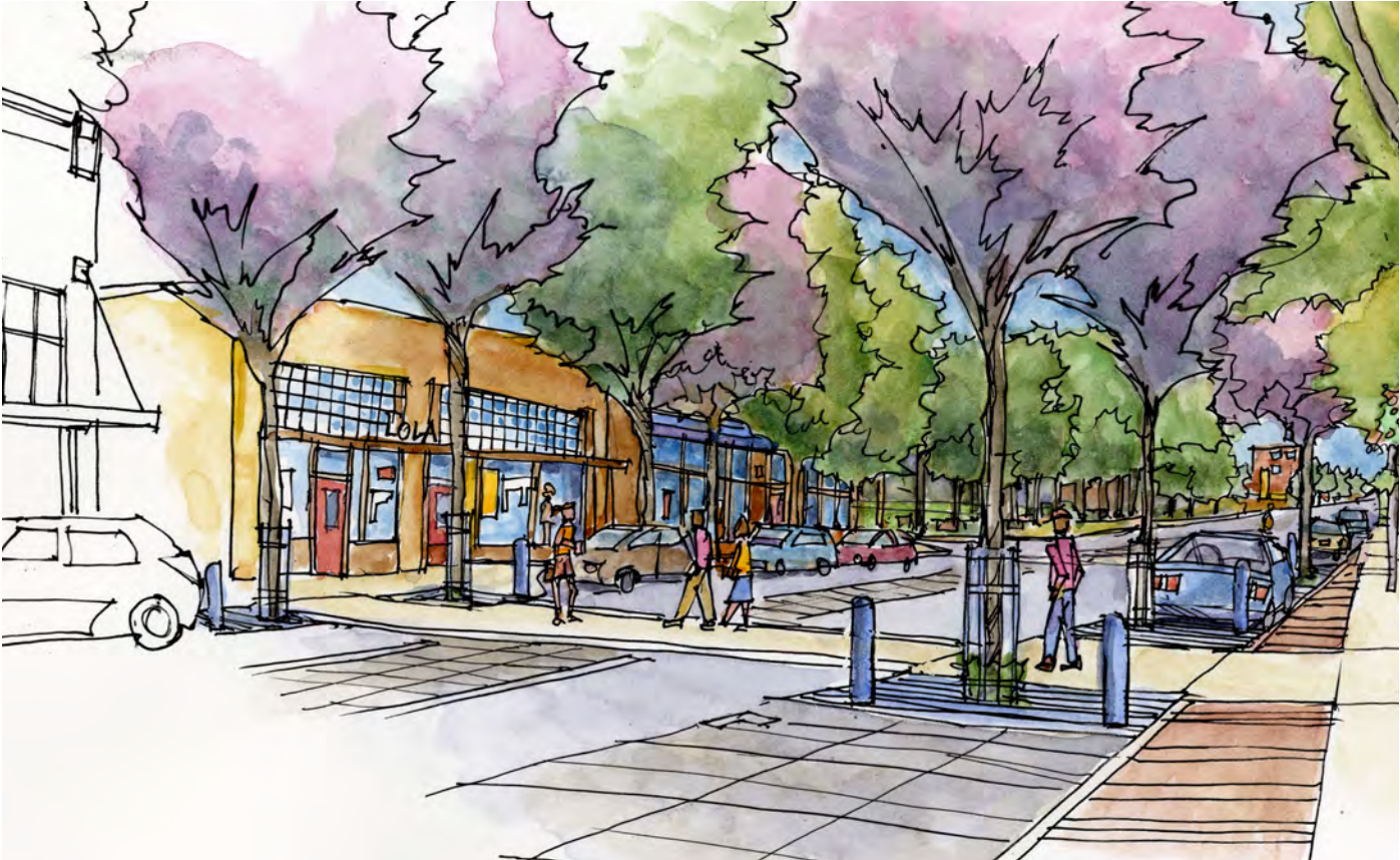
Figure 26: This sketch illustrates how a road diet and intermittent street trees and pervious paving in the parking lane can improve the street's visual character, narrow the street's real and perceived width to calm traffic, and increase green infrastructure opportunities. The bulb-outs and mid-block crossings would shorten crossing distances and times, while landscaping and pedestrian-scaled lighting would provide a more inviting place to walk.
