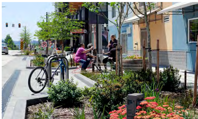
Figures E-1, E-2, E-3, and E-4: Bell Street is a shared street in a mixed-use area. Paving materials and colors, landscaping, and street furniture convey to drivers that this is a pedestrian zone and to slow down. (Image Credit: SvR Design Company)
