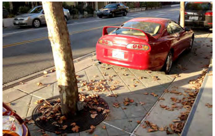
Figures A-7 and A-8: Trees in grated tree wells can provide numerous environmental and placemaking benefits. When placed in the parking lane, as on Castro Street in Mountain View, they create places that can be used flexibly for parking, seating, or community events. (Image Credit: Urban Rain | Design)
