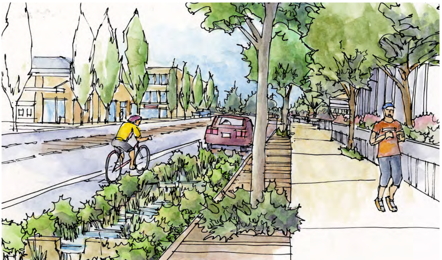
Figure 36: This perspective view depicts how a road diet and consistently planted street trees can increase safety and give the street more character. Reducing travel lanes and adding stormwater curb extension planters, permeable paving, and a bicycle climbing lane can work together to encourage downhill drivers to drive at a safer speed. Due to Capitol Way's gradient, stepping weirs (retaining walls that stormwater can flow over) can be used to slow the velocity of collected stormwater runoff and allow informational and playful art opportunities.
