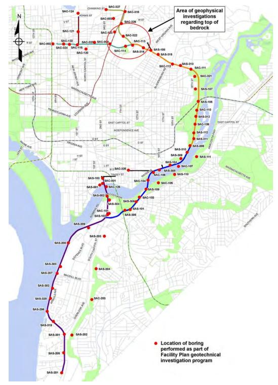
Figure 9: Locations of Borings and Geophysical Survey
