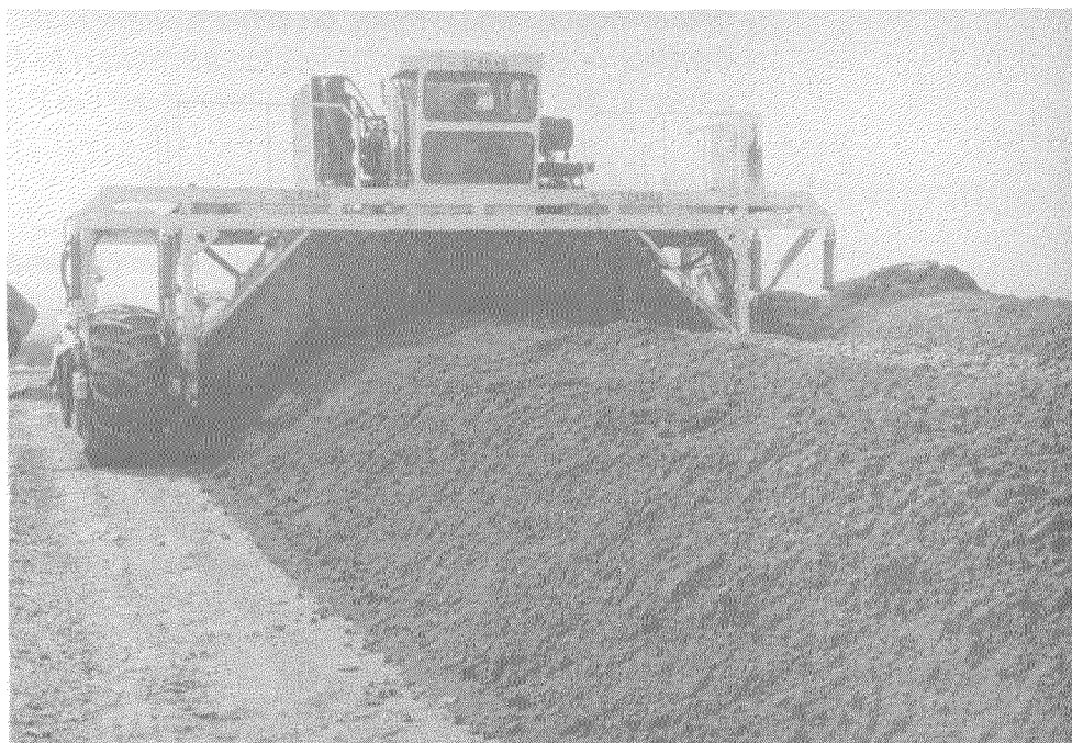
Open-air windrow composting operation near Los Angeles, California.
