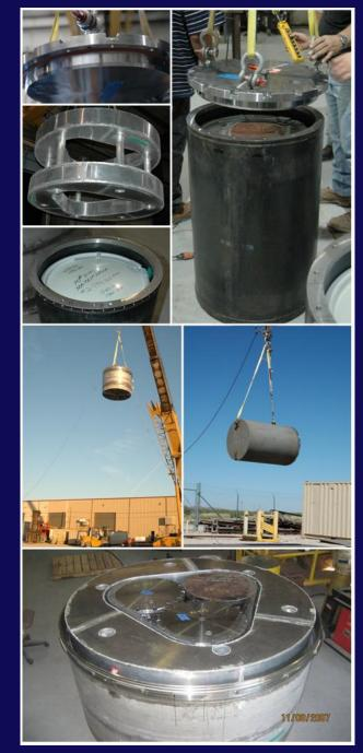
Shielded Payload Containers Will Enhance the Safety and Efficiency of DOE's Remote Handled Transuranic Waste Operations
