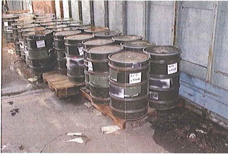
TNT Contaminated Water (red water/pink water)
