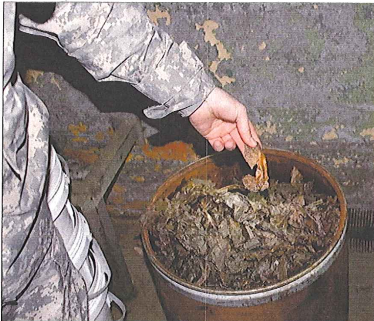
Tritonal scraps located in Building 1619 generated from Tritonal flaking operation
