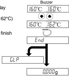
When the heater cover is opened during measurement or the STOP key is pressed, calibration is stopped and the analyzer displays the weighing mode.
