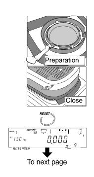
11. Open the heater cover. Put in a sample using the level indicator.
