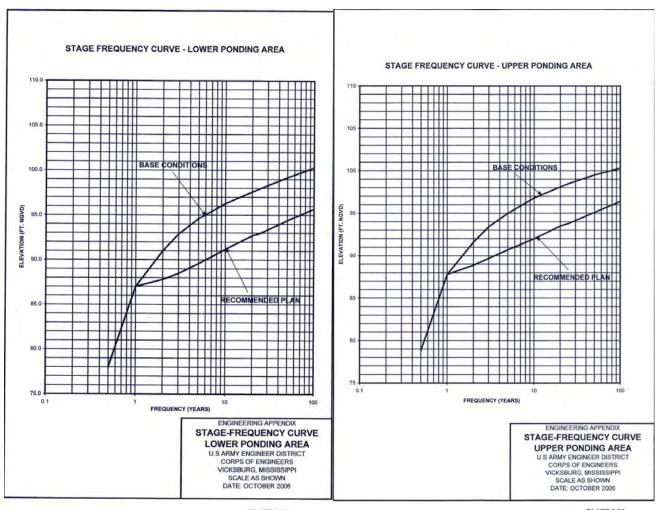
**Figure 2**. Plates 6-35 and 6-36 from the Engineering Summary of the Yazoo Backwater project FSEIS. Curves showing change in flood frequency in Upper and Lower Ponding areas as a result of the Pumps.
