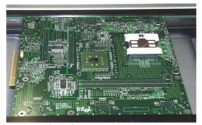
Figure 2. Reflow test PWB assembly
