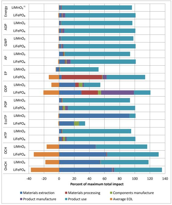
Figure 3. Life-Cycle Impact Assessment Results by Battery Chemistry and Stage for PHEV **Batteries**
