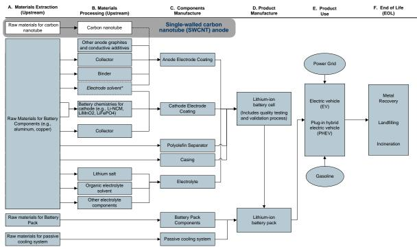
Figure 1. Generic Process Flow Diagram for Li-ion Battery for Vehicles
