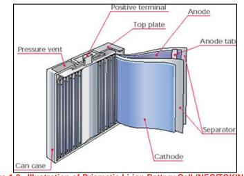
Figure 1-2. Illustration of Prismatic Li-ion Battery Cell (NEC/TOKIN, 2009)
