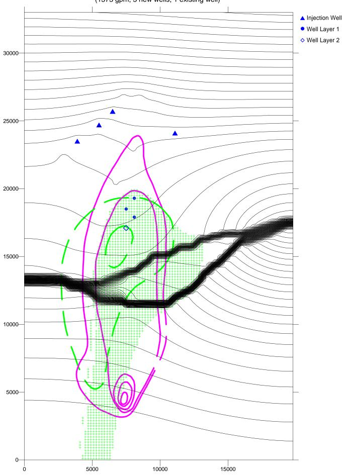
Figure 5-18: Shallow Particles, Contain Shallow 20-ppb Plume, & 500 gpm for Deep 20-ppb plume (1573 gpm, 3 new wells, 1 existing well)
