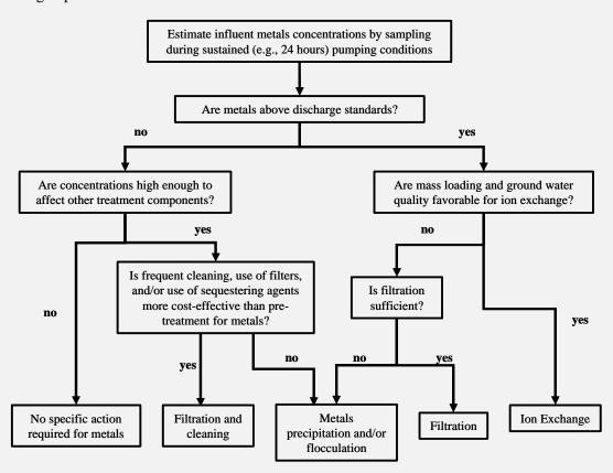
Evaluate costs for all options for each discharge location, and proceed with pilot test of most favorable option(s) as necessary. If metals precipitation or another large scale system is required, consider leasing equipment for several months to determine if problem is short-lived, or if a permanent system is required.
