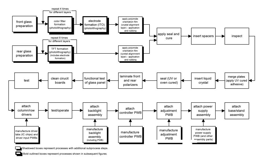
Figure 1-3. Traditional twisted nematic AMLCD manufacturing process
