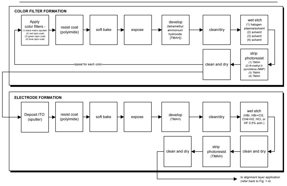
Figure 1-4. Front glass AMLCD manufacturing (photolithography)
