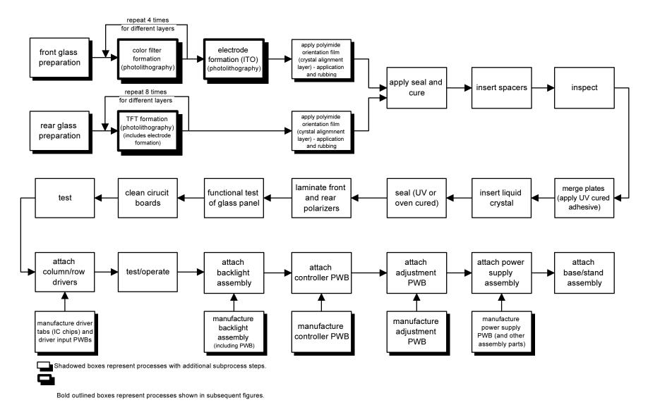
Figure 1-2. Traditional twisted nematic AMLCD manufacturing process
