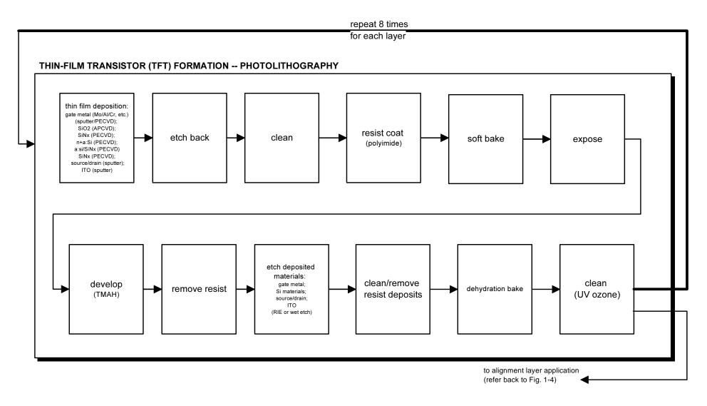
Figure 1-5. Rear glass AMLCD manufacturing (photolithography)
