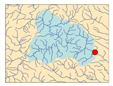
The blue shaded area is a Source Protection Area (SPA). Water from streams in the SPA will reach the intake in a 24-hour period. The red dot represents the intake.
