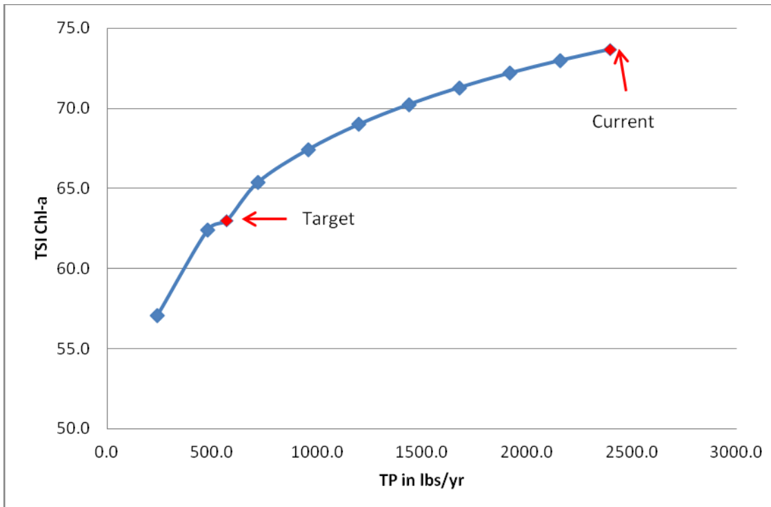
Figure E.2. The load response relationship between TSI Chl-a and total P as predicted by BATHTUB. The red square represents current conditions.
