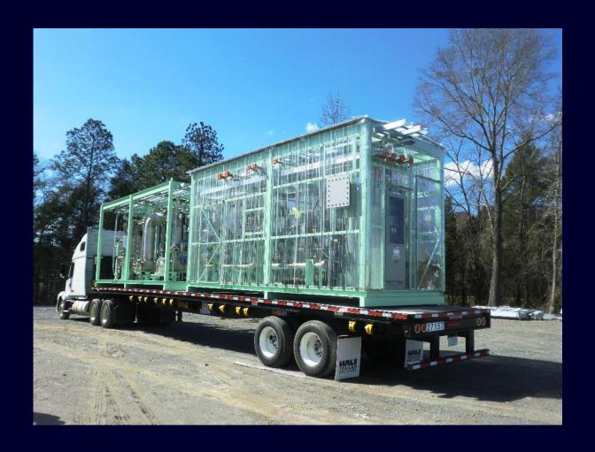
Assembled in 20ft. Standard Conex Frames
