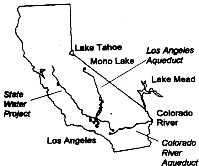
Figure 1-10. Sources of Imported Water in the Los Angeles Region (after Los Angeles Department of Water and Power, 1991).
