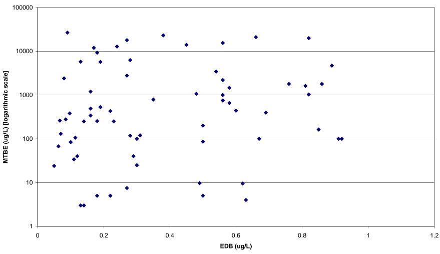
Appendix A-6, Figure 8: Groundwater Monitoring Results for EDB (1-100 ug/L) and MTBE
