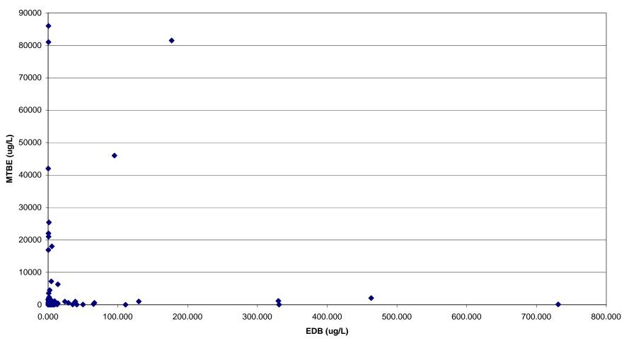
Appendix A-5, Figure 5: Groundwater Monitoring Results for EDB (<50 ug/L) and MTBE (73 data points)
