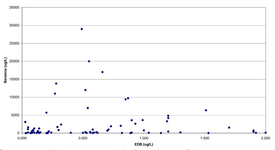
Each data point represents an individual groundwater monitoring sample (collected from a particular well on a specific date). Sources: (1) Analytical data for sites in California. Data available at https://geotracker.swrcb.ca.gov/. Accessed on August 26, 2004.
