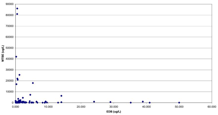
Appendix A-5, Figure 6: Groundwater Monitoring Results for EDB (<5 ug/L) and MTBE (53 data points)
