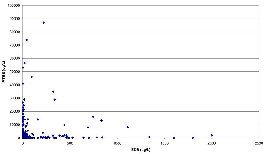
Appendix A-6, Figure 7: Groundwater Monitoring Results for EDB (<1 ug/L) and MTBE
