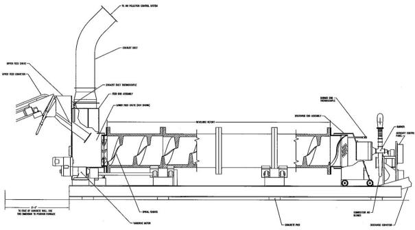
Figure 2: EDE's Rotary Kiln Incinerator for Explosive Wastes
