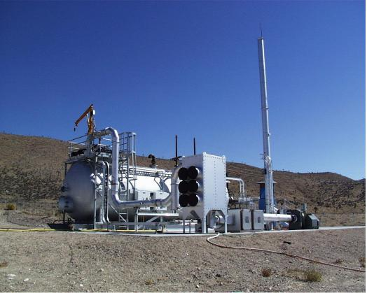
Nitrocellulose Based Propellant Contained Burn System Chamber and Pollution Abatement System
