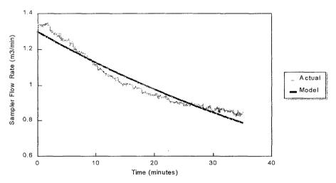
Figure 4.2. Sampler Flow Rate Versus Time.
