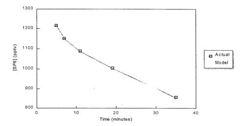
Figure 4.1. Concentration of SF<sub>6</sub> Tracer Gas Versus Time.
