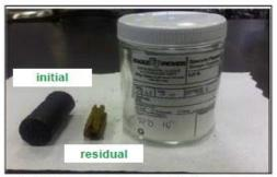
33g of NC propellant reduced to <5g of non-explosive residual in less than 48 hours
