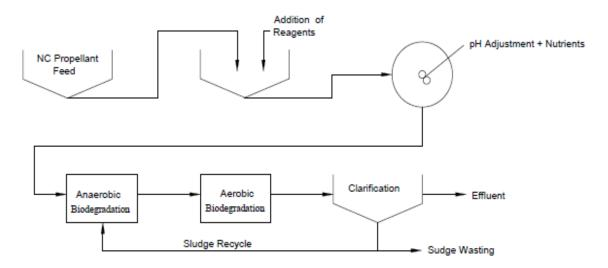
Flow diagram of NC propellant destruction with MuniRem proprietary technology and biodegradation process with denitrification (Adapted from USACERL TR-98/65)
