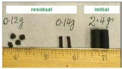
2.4 g of NC propellant residual in less than 24 hours of treatment
