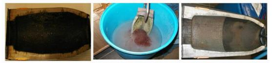
Rapid decontamination of halved bomb casings before and after MuniRem<sup>®</sup> treatment
