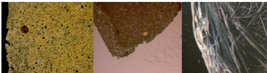
Figure 15. Appearance of M31 thin section exposed to water: (left) dark field view of yellow NC+NG and missing NQ crystals; (center) image showing wetting front and NQ crystals that formed from water; and (right) close up of NQ crystals.
