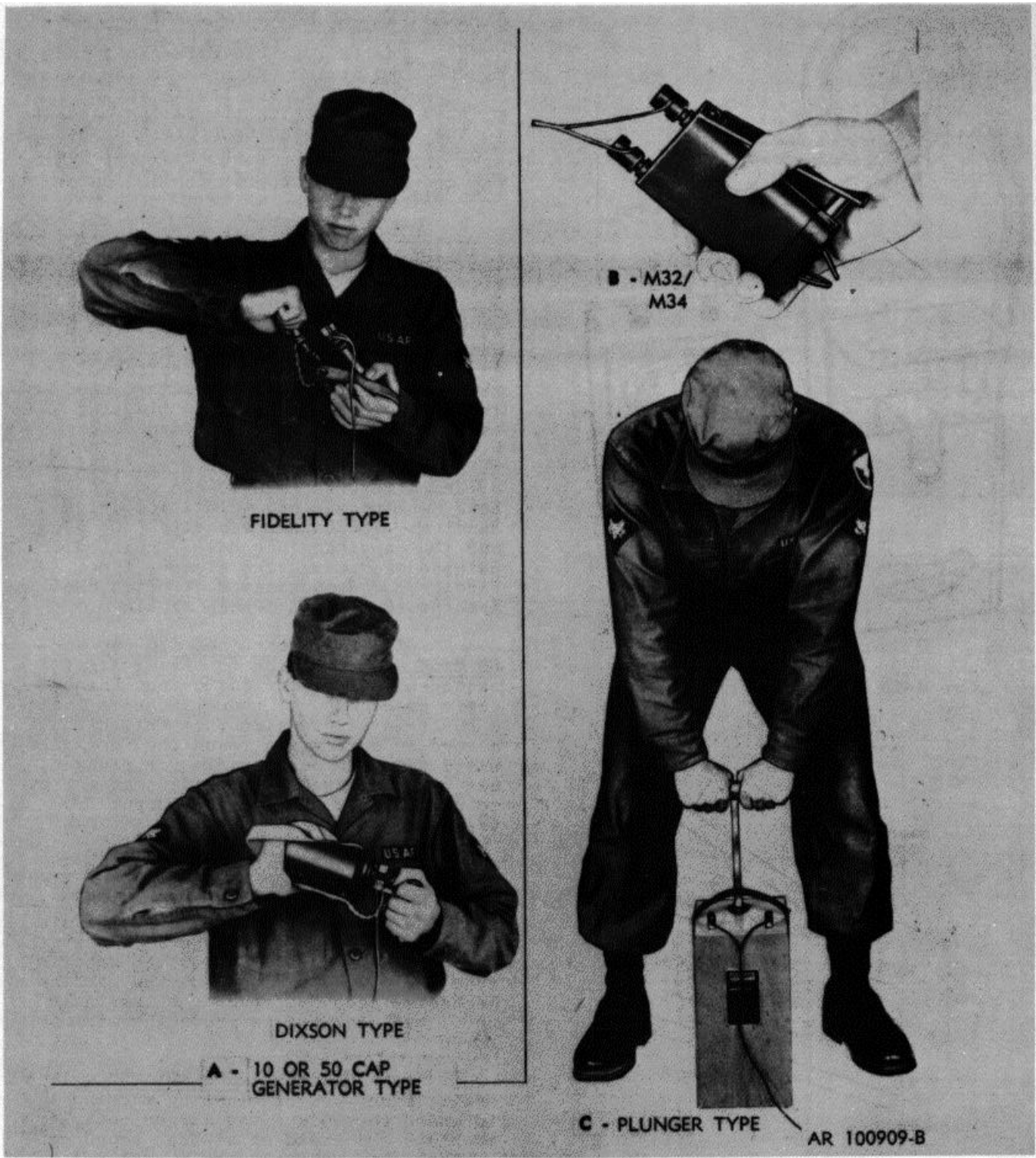
Figure 4-20. Actuating blasting machines.
