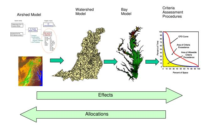
Figure A6: The CBP integrated models of the airshed, watershed, estuary water quality and sediment transport, key living resources, and climate change
