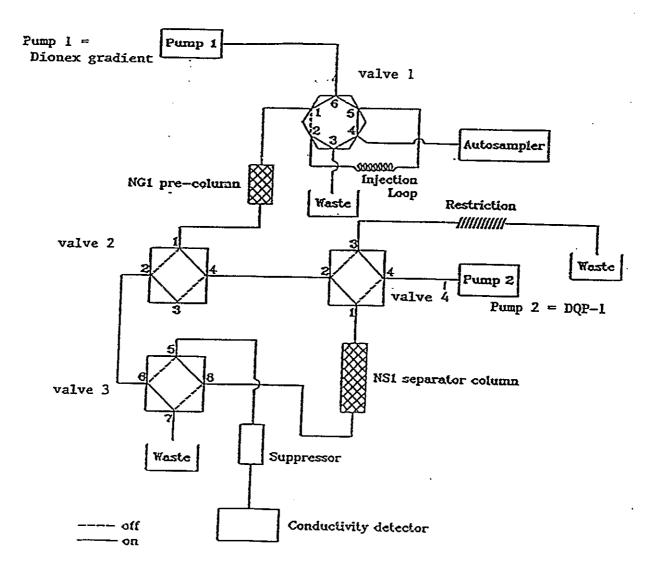
Figure 2. Suggested Configuration for the IC System.
