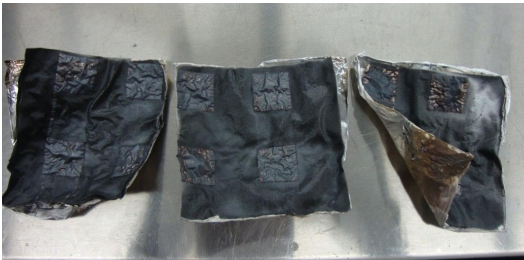
Figure 7-24. Final Chars for NFR Sample
