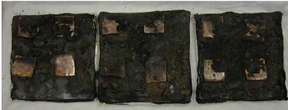
Figure 7-6. Final Chars for BFR + PHF Sample
