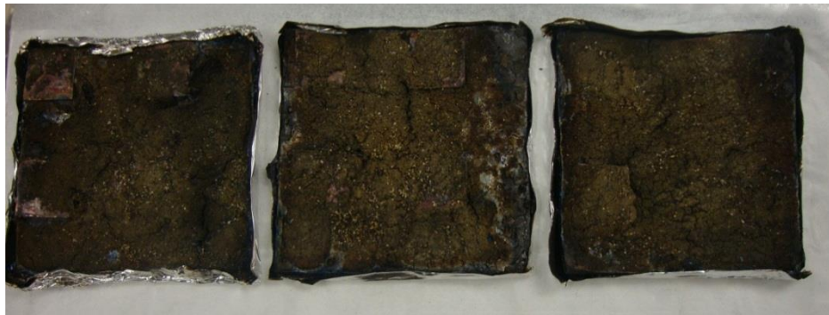
Figure 7-4. Final Chars for BFR + P Sample
