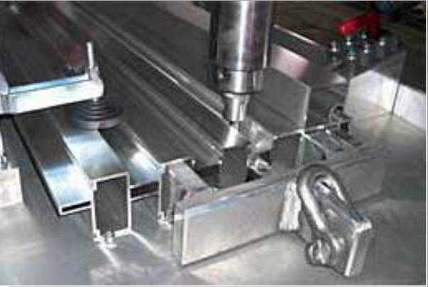
Low energy, low heat friction stir welding
